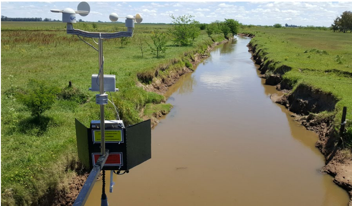
Waspote Plug & Sense! Smart Agriculture PRO measuring river level and weather parameters
